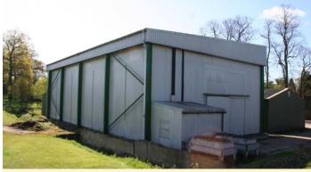
A modern steel portal frame purpose built cold store, that also comprises a secure storage facility, 3,319 sq ft GIA. Insulated walls and ceiling. Concrete floor. Power connected. Ceiling height - 6.42m. Sliding door - width 2.53m, height 3.17m.
