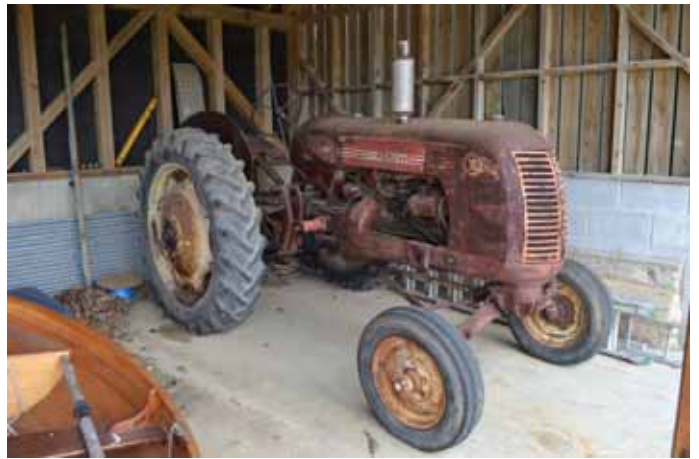
1. Cockshutt 30 petrol 2WD tractor. Model 4B153. Serial number 319921. 11-38 rear wheels and tyres. Electric start and swinging draw bar.
