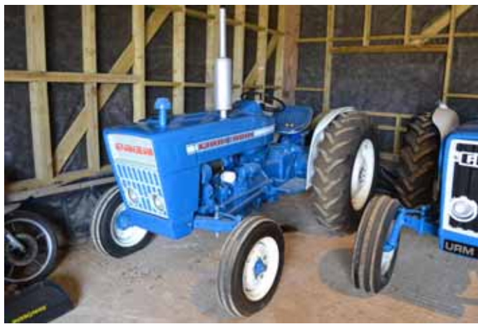
5. Ford 3000 diesel 2WD tractor. Serial number B931727. Showing 3921 hours. 14.9-28 rear wheels and tyres at 60%. Swinging draw bar.
