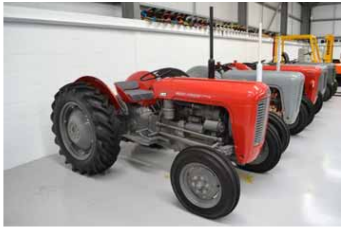
14. Massey Ferguson 35 Perkins 3cyl diesel 2WD tractor. 09/12/1959. Serial number SNM168839. Engine number 1801521. Registration 391 XUX. Showing 1001 hours. 12.4-28 rear wheels and tyres at 99%. Dual clutch and swinging draw bar.
