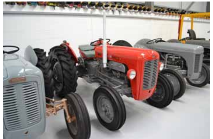
13. Massey Ferguson 35 petrol/TVO 2WD tractor. 09/02/1959. Serial number SKM129255. Showing 2403 hours. Registration SDL 839 (no paperwork). 12.4-28 rear wheels and tyres at 99%. Dual clutch and swinging draw bar.
