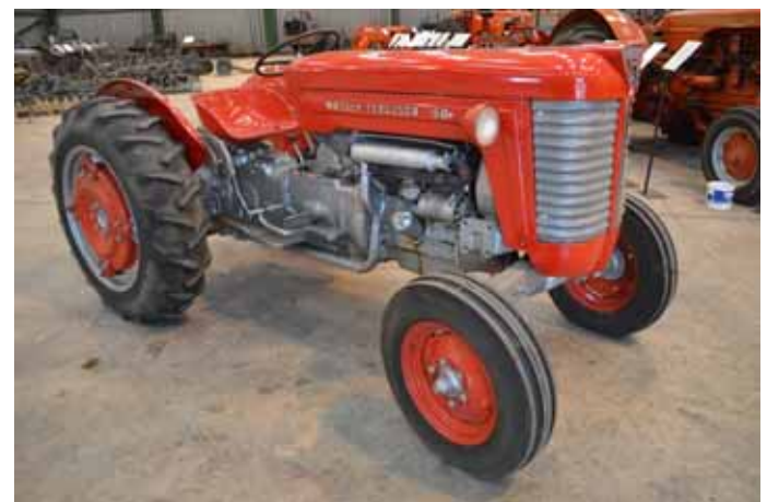
15. Massey Ferguson 50 petrol 2WD tractor. 1961. Serial number SGM528590. Engine number Z134711127. Registration 415 XUA. 12.4-28 rear wheels and tyres. Dual clutch and PAVT rear wheels. Ex-Hunday & Paul Rackham Collection.
