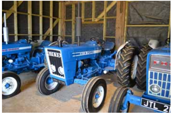
7. Ford 4100 diesel 2WD tractor. 1977. Serial number B989313. Registration URM 879S (incomplete paperwork). Date of first registration 17/11/1977. Showing 6981 hours. 14.9/13-28 rear wheels and tyres at 70%. Swinging draw bar.
