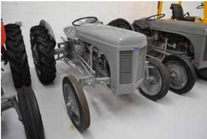
10. Ferguson TEA20 petrol 2WD tractor. 08/06/1948. Serial number TEA40357. Engine number S14184E. 11.2-28 rear wheels and tyres at 99%.
