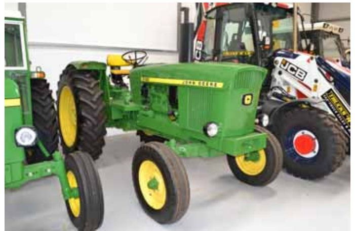
19. John Deere 3130 diesel 2WD tractor. Believed to be 1974/5. Serial number 142191L. Registration SCT 191N (no paperwork). Showing 849 hours. 16.9-38 rear wheels and tyres at 99%. Ex-Paul Rackham Collection and understood to have undergone extensive restoration by Ivan Cowlen.
