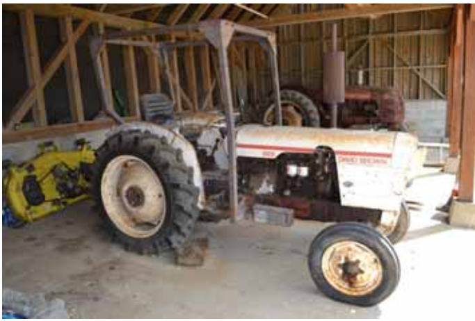
4. David Brown 885 vineyard diesel 2WD tractor. Serial number 885N/1 646317. Registration XER 740L (expired). Showing 1064 hours. 11.2-28 rear wheels and tyres at 80%. Swinging draw bar and roll frame.
